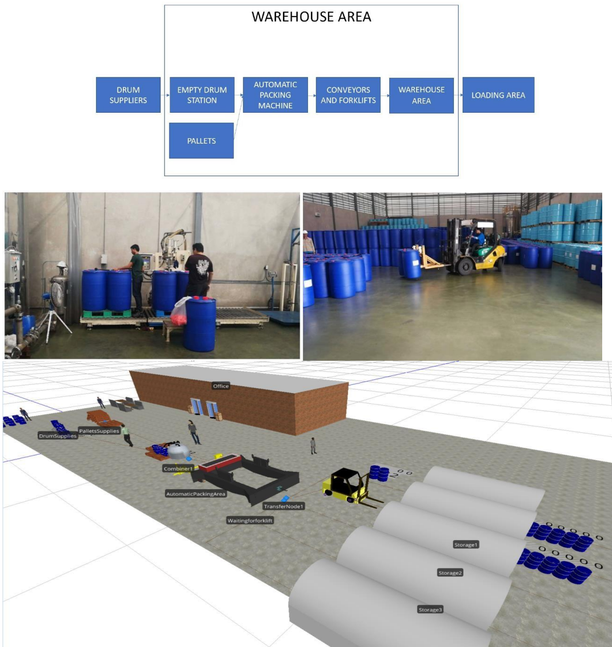
Figure 7: Rapid Prototype: Process Improvement – SIMIO Simulation Modeling
